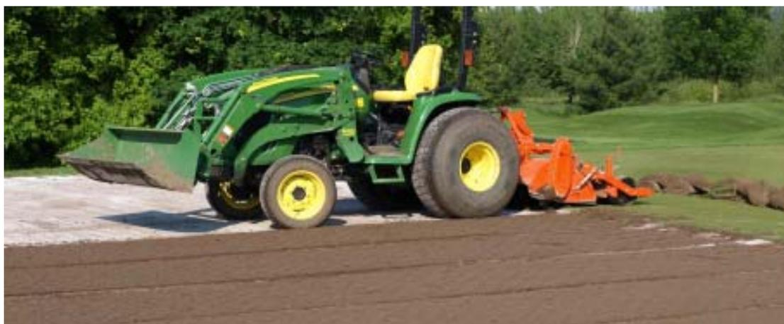
Figure 2. Incorporation of Basamid to 10 cm depth with Blecavator cultivator, June 15, 2011.
